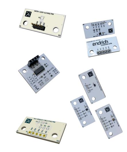
As new feature to extend the E-IoT platform, we introduced display solutions in a form of external boards based on different display standards such as pmOLED or TFT. These boards can be connected to either E-IoT SBC board or 3rd party MCU boards (Arduino, ESP32, Raspberry etc.) via standard interfaces.
