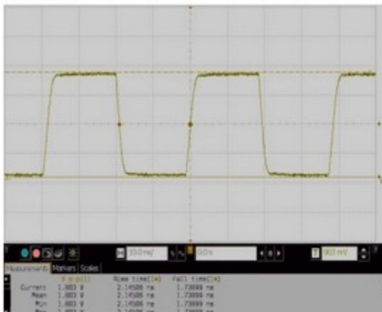
Fig. 13 Example of TST 26MHz XO Waveform
