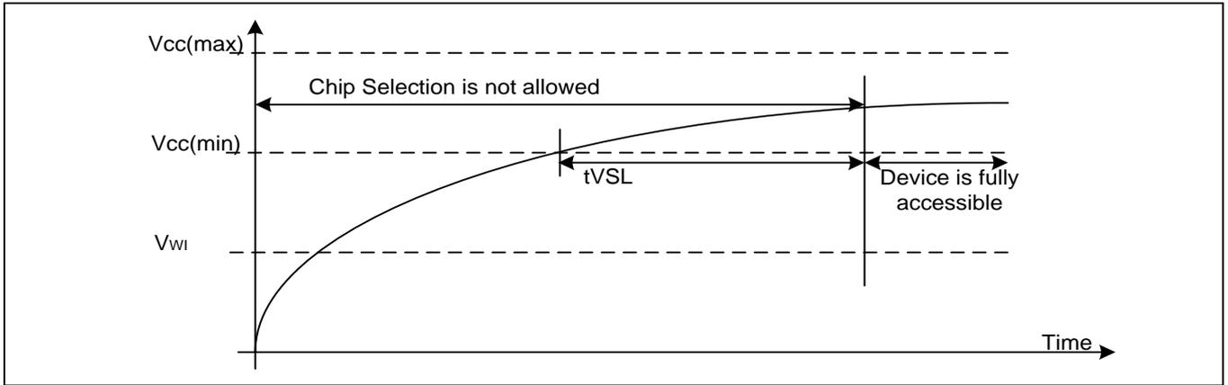
Table11-1. Power-On Timing and Write Inhibit Threshold for 1.8V/3.3V
