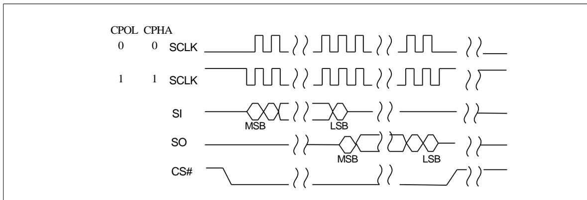
Note: While CS# is HIGH, keep SCLK at VCC or GND (determined by mode 0 or mode 3).
