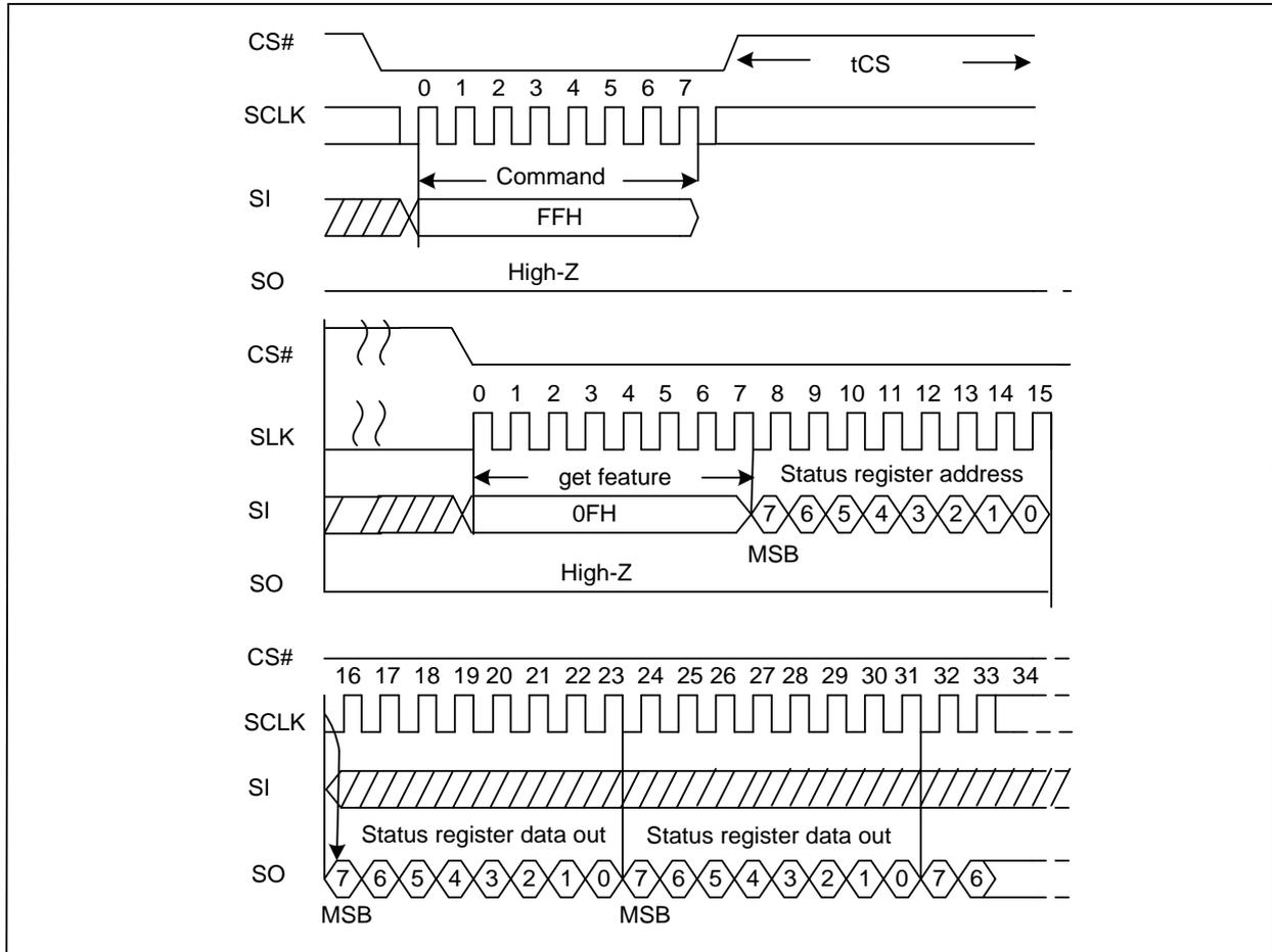
The RESET (FFH) command stops all operations. For example, in case of a program or erase or read operation, the reset command can make the device enter the wait state.
