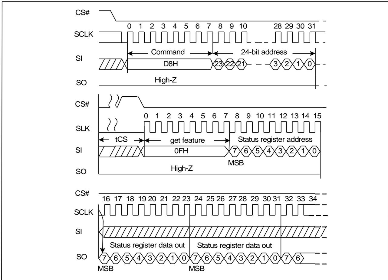
The BLOCK ERASE (D8H) command is used to erase at the block level. The blocks are organized as 64 pages per block, 2176 bytes per page (2048 + 128 bytes). Each block is 136 Kbytes. The BLOCK ERASE command (D8H) operates on one block at a time. The command sequence for the BLOCK ERASE operation is as follows:
