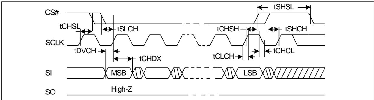
Figure26. Output Timing
